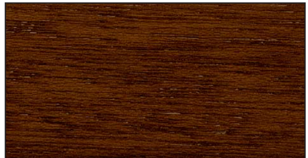
19 Species of wood: meranti Load group: B7/III-E Induline SW-900 clear Induline GW-360 wenge Induline LW-700/40 teak
