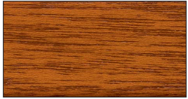
16 Species of wood: meranti Load group: B6/III-E Induline SW-900 clear Induline GW-360 teak Induline LW-700/40 cherry
