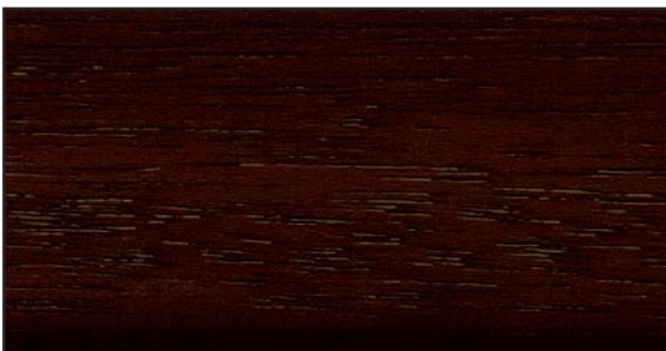
15 Species of wood: meranti Load group: B7/III-E Induline SW-900 clear Induline GW-360 wenge Induline LW-700/40 nut wood
