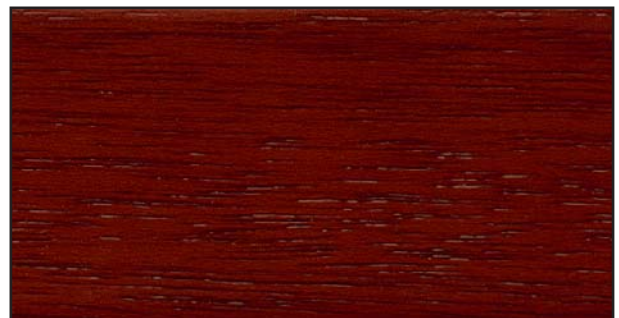
20 Species of wood: meranti Load group: B7/III-E Induline SW-900 clear Induline GW-360 teak Induline LW-700/40 mahogany
