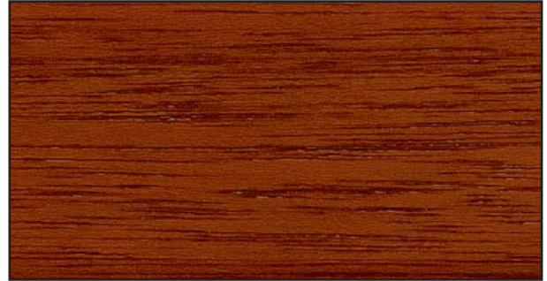
17 Species of wood: meranti Load group: B6/III-E Induline SW-900 clear Induline GW-360 teak Induline LW-700/40 teak
