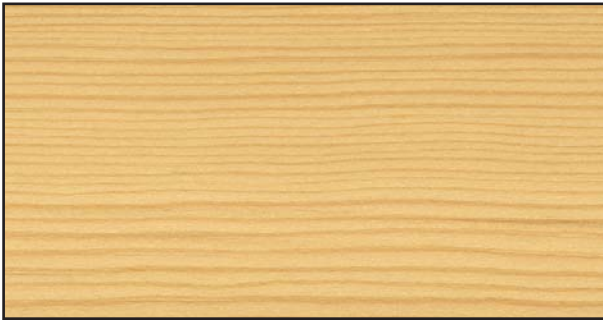
1 Species of wood: spruce Induline SW-900 VP 21087 Load group: Induline GW-360 clear - lignin stabilised B2/II-E Induline LW-700/40 VP 20181
