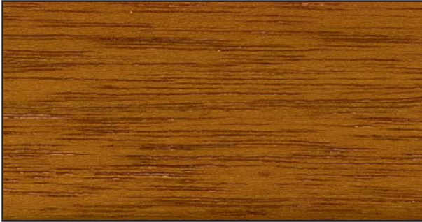
12 Species of wood: meranti Load group: B3/III-E Induline SW-900 clear Induline GW-360 teak Induline LW-700/40 chestnut
