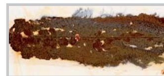
Salt spray test: No rust protection
