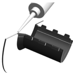
III. 3 – application of adhesive to the edges of the pipe flange
